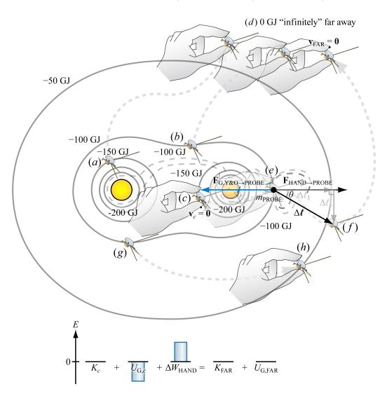
Fix the position of each object except for one and make a map of potential energy as a function of the position of this single moveable object.
